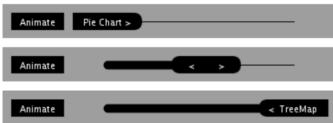
Fig. 9. The slider GUI, used in all interactive applets. It has a button to start and stop animating the morphing and labels to indicate the source and target visualizations — here, pie chart and treemap.
